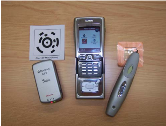
Fig. 4. Advanced mobile device including Wi-Fi, Bluetooth, GPRS/UMTS and camera (center), TRIP tag and Bluetooth GPS device (left) and RFID tag and Bluetooth RFID reader (right)
